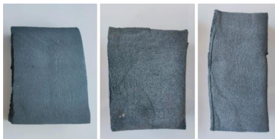
Figure 3: One RR Specimen for each 8 %, 12 % & 20 % FA reinforcement from left to right
